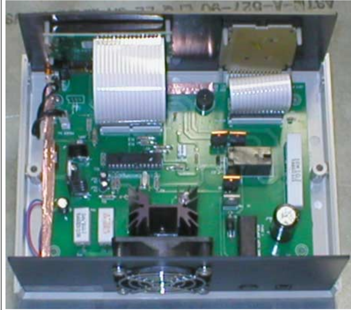
Figure 3: View of Controller PCB mounted in enclosure
